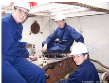
Trainees assist with the removal of the cylinder covers (Port Main Engine)
