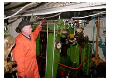
John Deakin inspects a cleaner starboard engine following the October cleaning operation.
