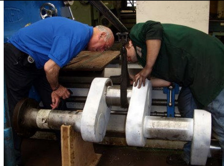
Daniel Adamson Engine Crankshaft Undergoing Examination photo: Mike Williams
