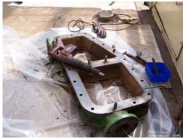
The port condenser, forward water box dismantled for cleaning, once again our faithful 'Hilti' needle gun is used to good effect.
